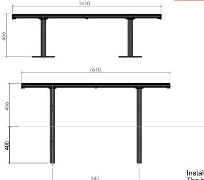
BACKLESS BENCH ASSEMBLY INSTRUCTIONS Turn the bench upside down, being careful to protect the wooden parts during installation. Using a screwdriver with an H6 bit, secure the supporting post to the underside of the seat with the screws and washers included (MK6S M10 x 16 + FBB M10).
