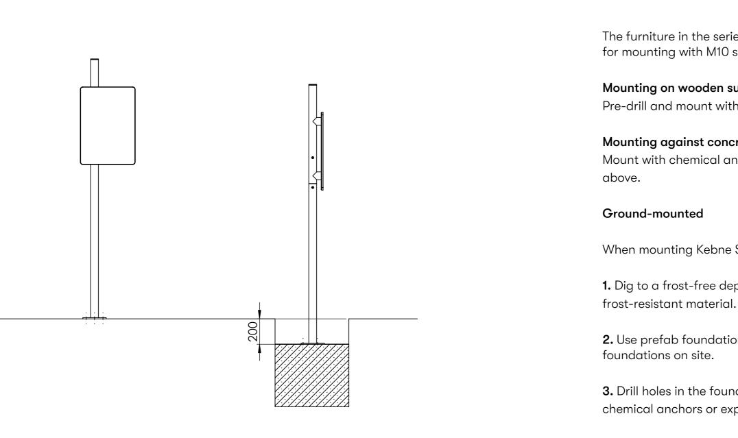
4. Finally, fill in about 200 mm with shock-absorbing substrate. For example, bare soil, gravel or sand.
