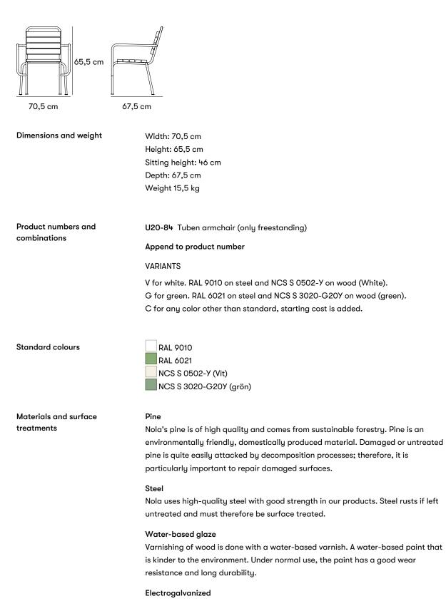
Electrogalvanizing (also known as zinc plating) provides corrosion protection through the sacrifice of zinc ions. It is created via a zinc coating on the steel using an electric current.
