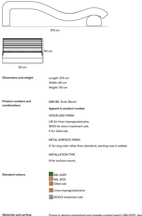
Frame in electro-galvanized and powder-coated steel in RAL6025, gloss 70. Slats in pine or oak.
