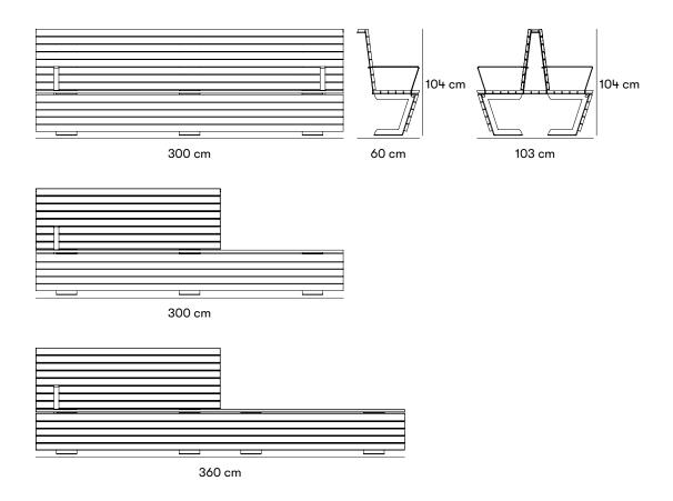
Dimensions and weight U19-50 Single sided Backed bench Length: 300 cm Width: 60 cm Height: 104 cm Seat height: 44 cm Armrest height: 67 cm Seat depth: 43 cm 3 frames C-C frames: 120 cm
