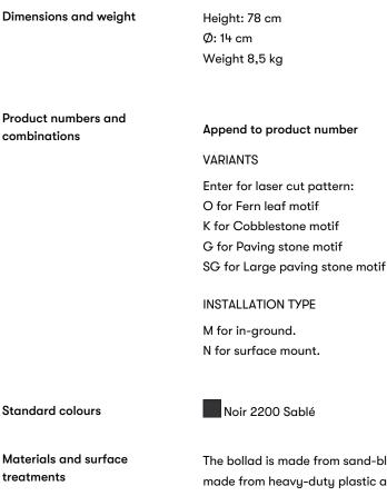
The bollad is made from sand-blasted, chromated steel pipe with an inner pipe made from heavy-duty plastic and a reflective foil on the surface. The bollard is powder-coated in standard colour black Noir 2200 Sablé.
