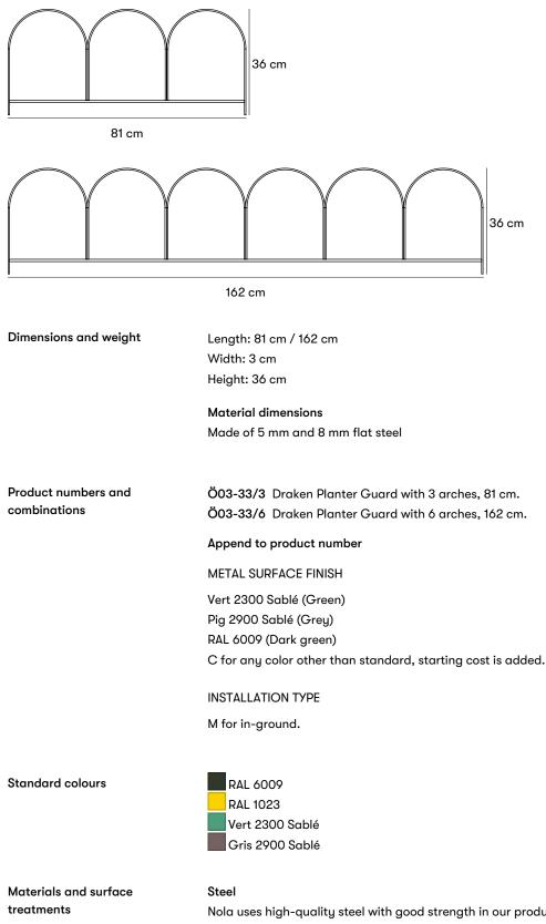
Nola uses high-quality steel with good strength in our products. Steel rusts if left untreated and must therefore be surface treated.
