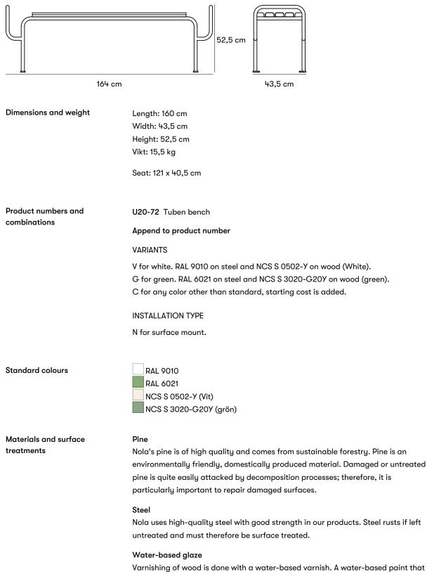
Varnishing of wood is done with a water-based varnish. A water-based paint tha is kinder to the environment. Under normal use, the paint has a good wear resistance and long durability.
